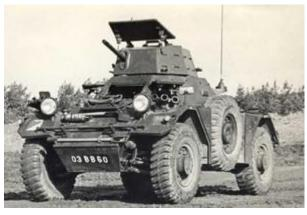
The Ferret Scout Car was of British origin and was armed with a .30 cal Browning machine gun, a six cylinder Rolls Royce petrol motor, weighed 3.75 tons, could reach speeds of 60 mph and had a crew of two. The Ferret Scout Car was first used in the Regiment around 1958 and there were two models the MK1 which had no turret, the MK2 which came along later fitted with a turret.
