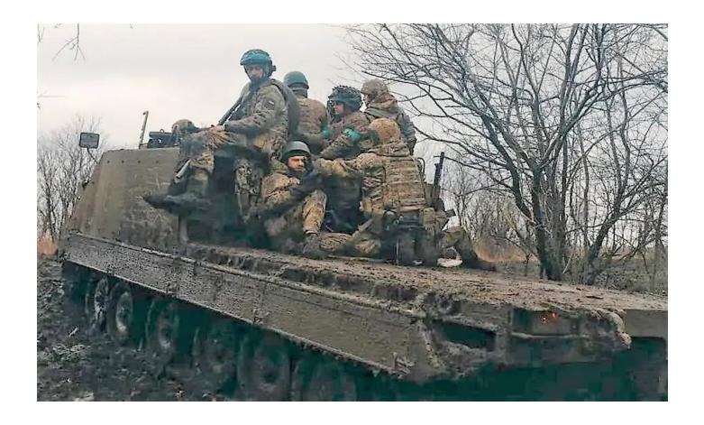
The M113AS4 APC, an upgraded version of the M113AS1 used during the Vietnam War, has undergone various improvements in its systems. These enhancements include a new engine, with the Australian M113AS4 equipped with an MTU 6V 199 TE 20 engine, enabling the vehicle to reach speeds of up to 66 km/h. Additionally, the steering controls, drivetrain, electrical systems, and fuel systems have been revamped. The M113AS4 has an impressive travel range of up to 550km.
